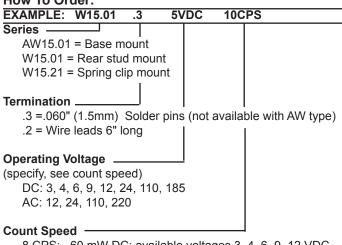
8 CPS: 60 mW DC; available voltages 3, 4, 6, 9, 12 VDC 10 CPS: 500 mW DC; available voltages 4, 6, 12, 24, 110, 185 VDC
