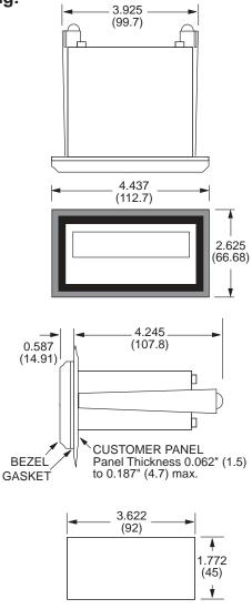
**NOTE:** Allow an additional 0.75" in depth when using the "PC90PT" series ribbon adaptors
