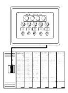
The MMI-700 uses each PLC's communication protocol to read or write data. It does not require the PLC to run any special program for data communication, which greatly reduces programming time. The available PLC drivers include A-B, Siemens, Omron, MITSUBISHI, Aromat, Koyo and GE Fanuc, etc. More and more supporting device drivers are being developed every day. The MMI-700 uses dynamic
