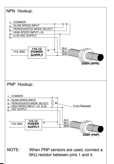
Our D Series Proximity Sensors interface easily with our full line of counters and ratemeters. Use PNP sensors (D\_P) on all KEP units except KAL Series, which requires D\_N (NPN) sensors. (See Sensors & Accessories Section)
