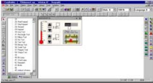
Graphics can be produced by using the EasyBuilder's own set of drawing tools. You can import any 256 color BMP format graphic into EasyBuilder to customize your application. Screen Captures and Graphics may also be cut and pasted into Paintbrush for conversion to the BMP format. Libraries with over 300 commonly used graphics are included with EasyBuilder Software. These libraries can be edited and new libraries created to hold new graphics you have created.
