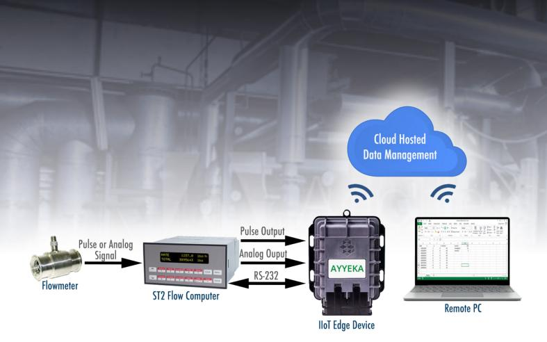
Move your flow computer data to the cloud using an Ayyeka Wavelet device and access the information from a remote PC or mobile device. The Ayyeka cloud service is secure and private. The web-based data management system enables you to configure the device over-the-air and program various parameter threshold levels for email and/or SMS alerts, visualize data in real-time, and produce reports for presentation and analysis
