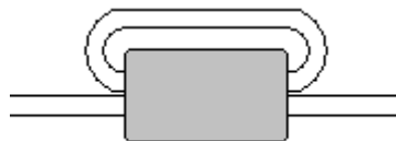
140 \Omega @ 100MHz ferrite
