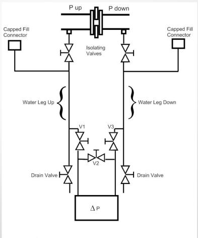
$\Delta P = (Pup + Pwater leg up) - (Pdown + Pwater leg down)$
