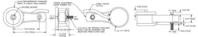
Note: All dimensions are in inches (mm) with a tolerance of +0.005" or +0.01" unless otherwise specified.
