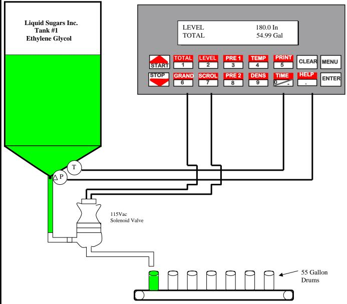
The Leveltrol II has the ability to perform in bulk fluid transfer applications. It uses an internal register to keep an audit trail of instrument set up changes.
