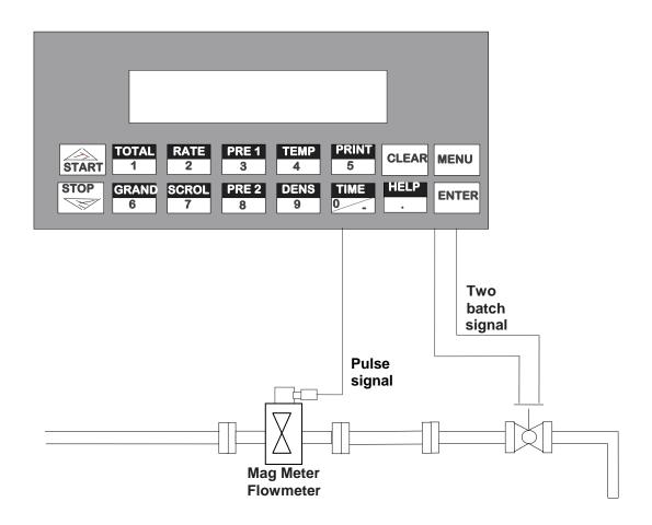
The SUPERtrol-1LE has the ability to perform in custody transfer applications. It uses an internal register to keep an audit trail of the number of instrument set up changes.
