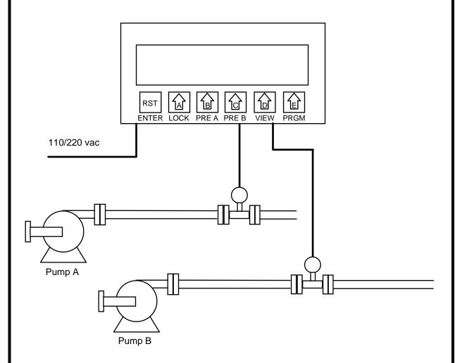
The MINItrol MRT powers both turbine flow meters and accepts their pulse input signals on channels A and B. In this application the MINItrol is programmed so as to add together the pulses from channels A and B (A+B mode). In this way a total consumption of additive is calculated.
