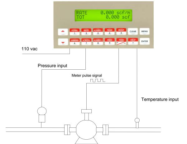
The SuperTROL-II utilizes the pressure and temperature signals, as well as user input data, to compute the density of the flowing natural gas. The SuperTROL-II then performs a calculation that is referenced to standard conditions. The result of the calculation is displayed in SCFM or NM<sup>3</sup> per hour and totalized in SCF or NM<sup>3</sup>.
